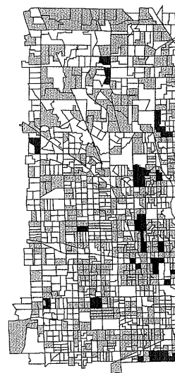
Figure 9-19: An example of a dissolve operation. Note the removal of lines separating polygons of the same size class. This greatly reduces the number of polygons.
