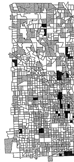
Figure 9-17: Natural breaks classification. Boundaries between classes are placed where natural gaps or low points occur in the frequency distribution.
