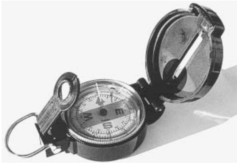
FIGURE 2 A Simple Compass for Measuring Angles
